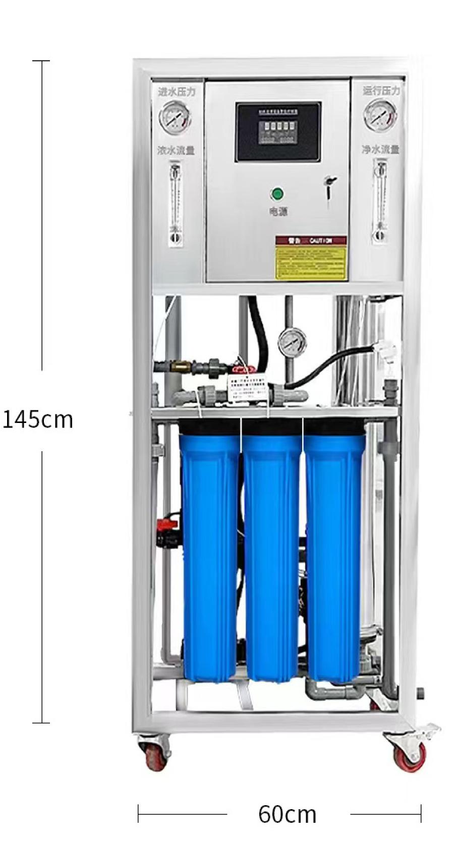
Body size: 60\*60\*145cm Weight: 57kg Body material: stainless steel Power supply: 220V Power: 1.1–1.5kw Applicable water 02. -0.5Mpa pressure: pplicable water ≤ 1200ppm source: Working 0 ℃ - 38 ℃ environment: Water 0.5T/Hproduction: MR brand Booster pump: RO membrane: MR brand 6 PCS 20 inch filter Filter: valve head: manual/automatic PVC pipe/stainless steel pipe pipeline: Electrical parts: Delixi/pure copper solenoid valve
