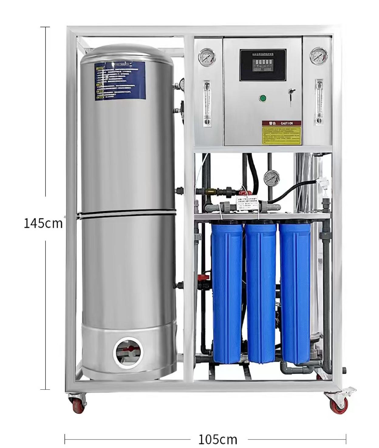
105\*60\*145cm Body size: Weight: 77kg Body material: stainless steel 220V Power supply: Power: 1.1-1.5kw Applicable water 02. -0.5Mpa pressure: Applicable ≤ 1200ppm water source: Working environment: Water 0.5T/Hproduction: Booster pump: MR brand RO membrane: MR brand 6 PCS 20 inch filter Filter: valve head: manual/automatic pipeline: PVC pipe/stainless steel pipe Electrical parts: Delixi/pure copper solenoid valve
